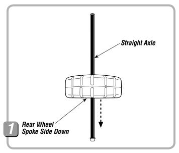
• Slide a rear wheel (spoke side down) onto the straight axle.
